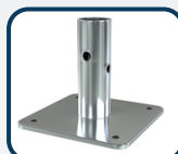
BASE PLATE Standard : EN74 / BS1139 Size : 150mm * 150mm * 6mm Finish : HDG
